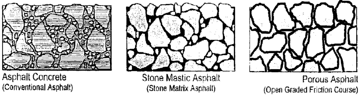
Figure A6-12. Asphalt concrete vs SMA vs porous asphalt
