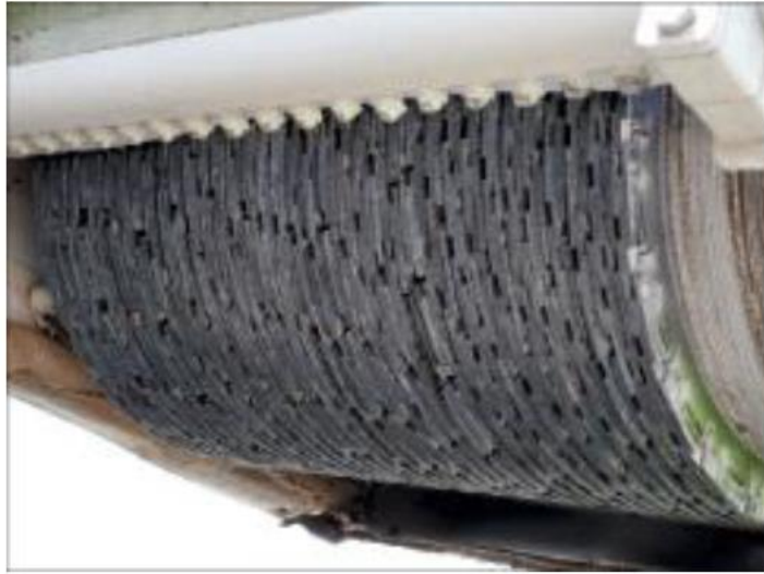
Figure A6-8. Diamond grinding of cement concrete
